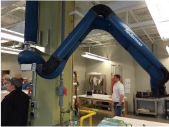
PORTABLE DUST COLLECTION PICK UP ARMS CAN BE MODIFIED FOR ELEVATED TEMP OPS LOCATE ON SUPPLY PLENUMS TO DIRECT ONTO HULL INTERIOR SPACES
